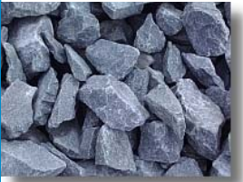
Use angular rock (above) or river rock (below) for bridge approach.
