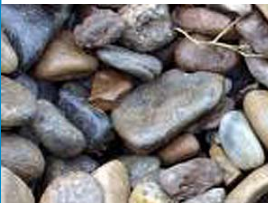
Use angular rock (above) or river rock (below) for bridge approach.
