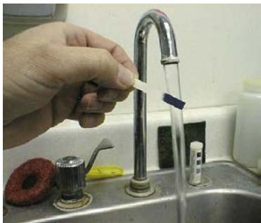
► Turn on the power to the pump. Run chlorinated water through the entire plumbing system by running water to each fixture\* one at a time until you smell bleach (or use chlorine test papers available at pool supply businesses) and then close the fixture. Do this for each fixture, including:
