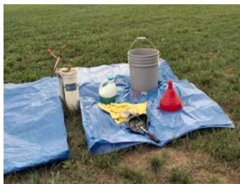
Do not place well components directly on the ground.
