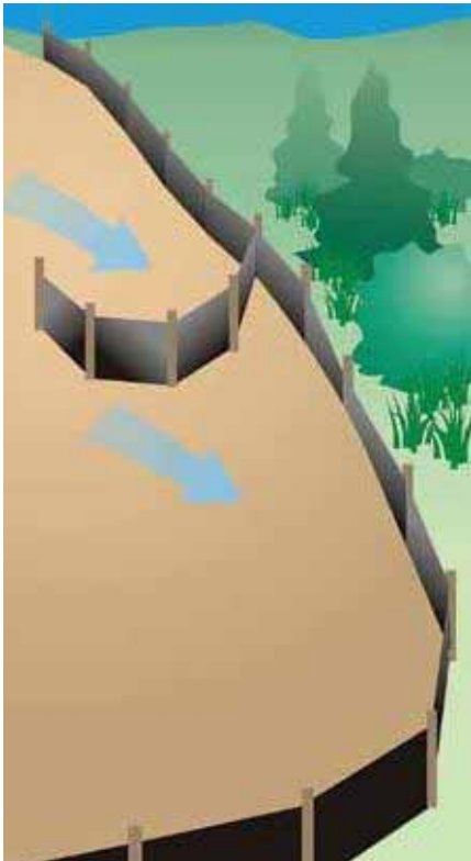
Curve the ends of silt fence and other sediment controls up slope to form a "J-hook".
