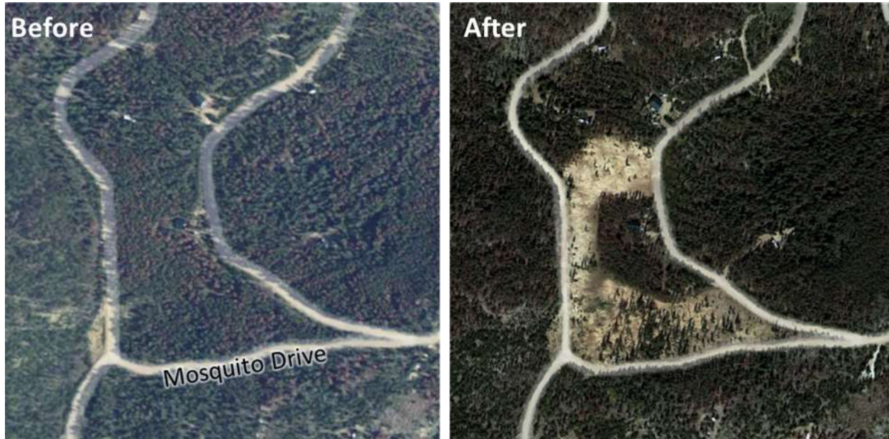
Figure 4.d.1. Effective roadside fuel treatments remove enough trees to result in widely spaced crowns, remove ladder fuels, and reduce surface fuels. More dramatic tree removal along roadways can create even safer roadway conditions where appropriate. Photo credits: Genesee Foundation (left) and USDA/FPAC/GEO/Google Earth (right).
