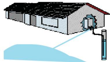
**Open-loop system.** During winter, ground water is drawn from a well to the heat pump for "once-through" use, then discharged to a pond (shown above), onto land, or into an injection well. This system may require one or more permits from DNR or other agencies. Regular maintenance may be needed to descale the heat exchanger, or installation of a higher cost heat exchanger resistant to corrosion may be needed.
